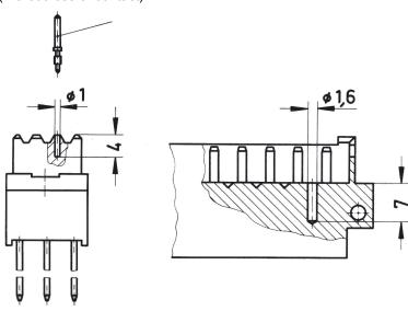
To avoid cross-plugging of adjacent connectors a coding system is required.
